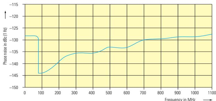
Typical SSB phase noise versus carrier frequency
