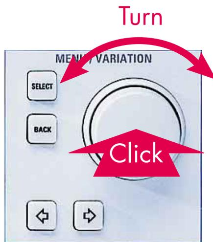
Simply select the desired menu with the spinwheel and click the button to open the submenu
