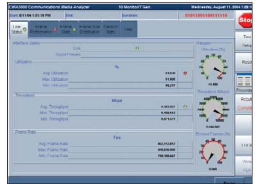
With the press of a single button, important network parameters such as link status and utilization may be obtained. In addition, unmistakable alarm notification will signal compromised network performance when service degrades below any one of 15 preset, user-defined thresholds.
