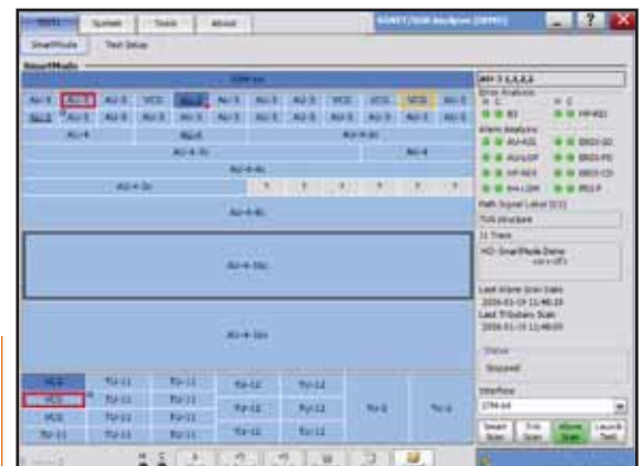
FTB-8120/8130 SmartMode: multichannel signal discovery with real-time alarm scan (shown in the FTB-400 user interface).
