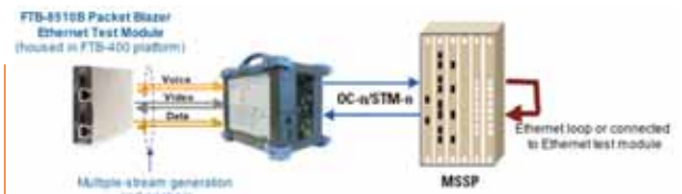
Combining the FTB-8510B's Ethernet multiple-streaming capabilities and the FTB-8120NG/8130NG embedded Ethernet interfaces creates a powerful solution for testing multiple services over SONET/SDH.
