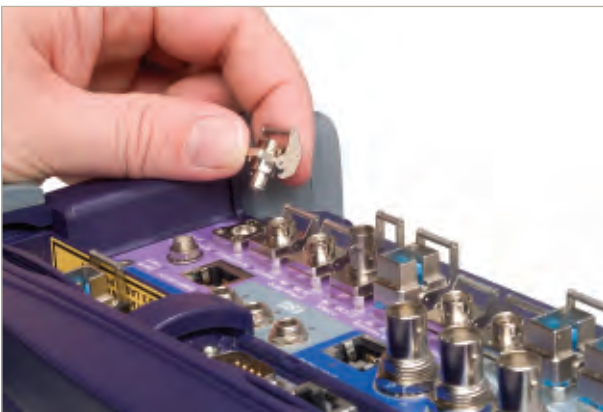
Field exchangeable optical connectors
