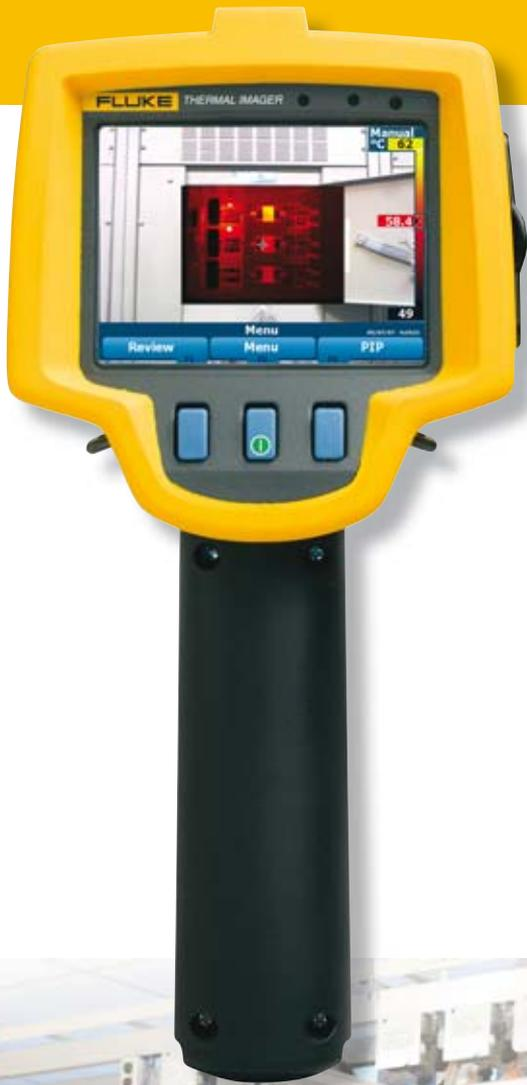
**Palette**—Color representation of the temperatures (temperature scale) in a displayed image. Certain color palettes meet personal preferences or optimize the image for different applications and/or problems. An example of the different palettes appear to the right.
