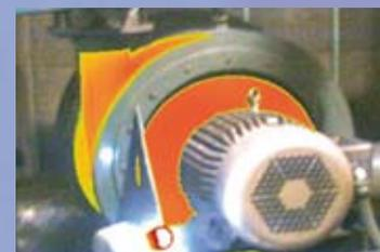
**IR/Color Alarm** Displays only temperatures falling above, below, or in between a user-selected range in infrared, and anything outside the selected range as a visual (visible light) image. (In software only.)
