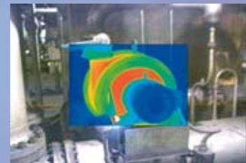
**Picture-in-Picture** Creates an IR 'window' surrounded by a visual (visible light) frame to easily identify problems, while maintaining a frame of reference with surroundings.
