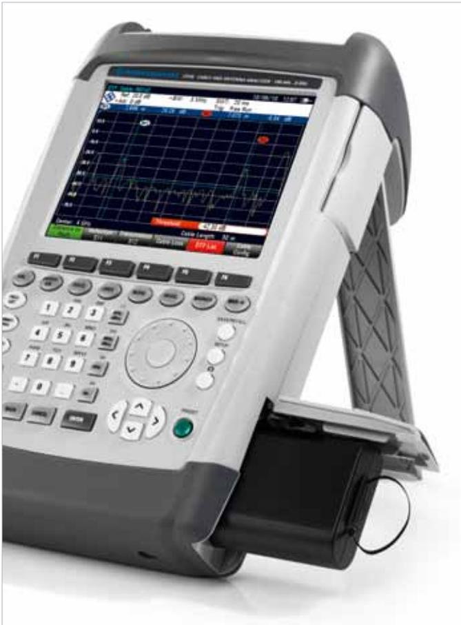
Easy-to-replace Li-ion battery for up to 4.5 h of operation.
