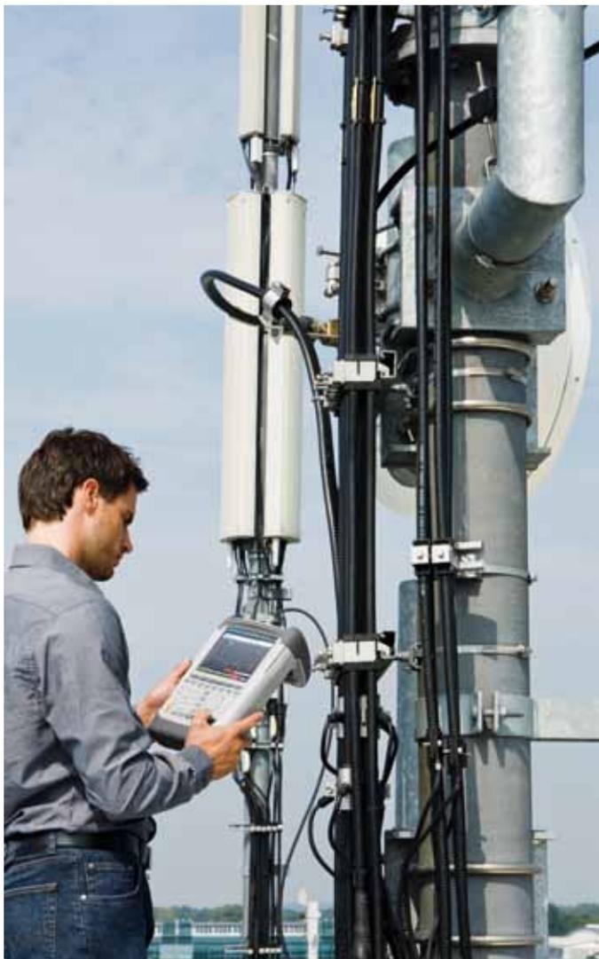
Distance-to-fault measurement at a mobile radio antenna system with the R&S®ZVH.
