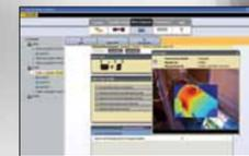
**Viewer PC Software** expands data storage and tracking capacity and imports Fluke thermal images
